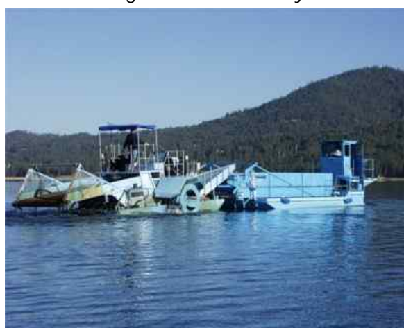
Harvester off-loading to the transporter
