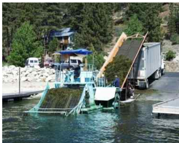
Harvester off-Loading to the Conveyer Belt
